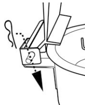
lock the bar with a pin
